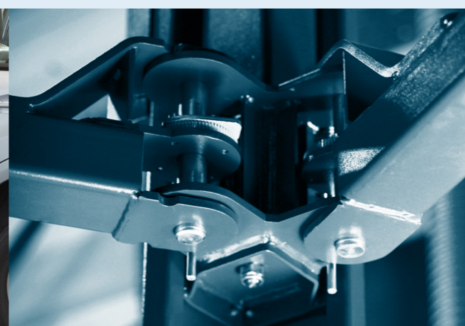
Automatic locking of lifting arm
