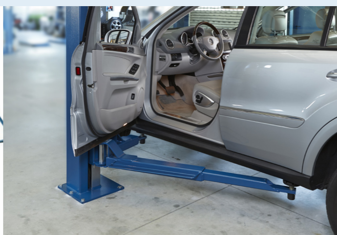
Optimal door clearance with asymmetric arms
