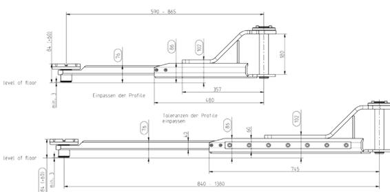
SC (Sports car arms): extremely flat construction. Very sturdy, made of solid material. Especially suitable for very low and wide sports cars.
