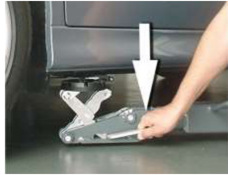
Figure 2: If required, place the carrier plate by pushing the lever at the fixture points
