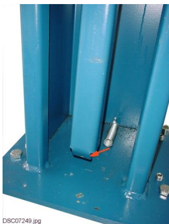
pic 6: Hang the spring into the ratchet-strip
