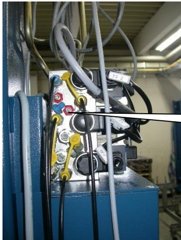
Figure 8: Loosen both red locking nuts on the hydraulic block. Afterwards, loosen both emergency discharge screws using an Allen key (size 5) by a maximum of 1 rotation anti-clockwise.
