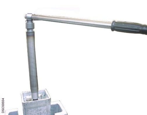
Figure 9: Screw on the long threaded sleeve (available from your dealer) and tighten clockwise using a suitable tool (spanner width 24) Lower the lift rails approx. 5-10 cm. Repeat the process on the next lift rails etc. The lift rails may only be lowered in steps of 5-10 cm until the entire lift has reached the lowest position.
