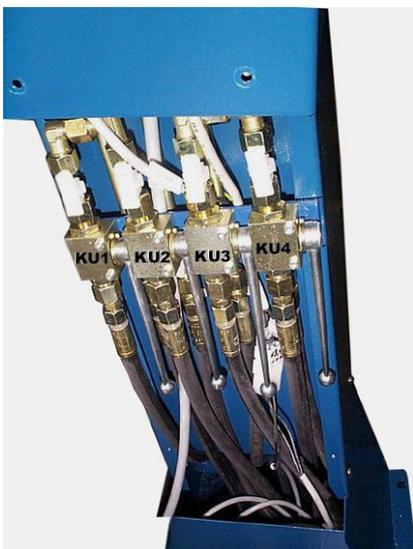
pic. 2: ball valves for the equalization of the lift.
