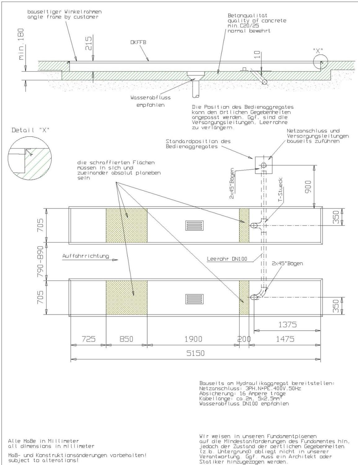
Fundamentplan UNI-LIFT 5000 NT PLUS
