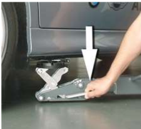
Figure 2: If required, place the carrier plate by pushing the lever at the fixture points.
