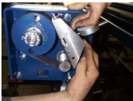
Figure 17: Place the dial gauge on the belt
