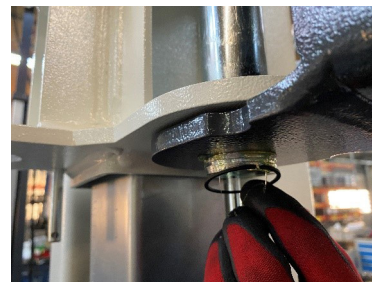
Fit lower circlip to pin
