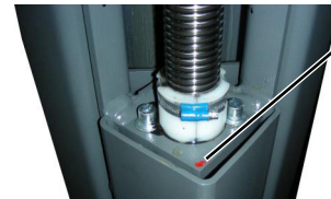
Figure 18: The lift nut pin is provided with a sealing wax
